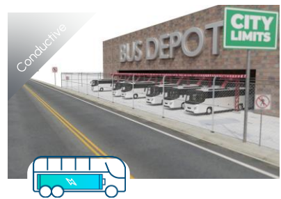
Overnight conductive (plug-in) charging
